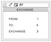
Press P+/- to select the item and then V+/- to adjust the channel and V+ to confirm.(For example: press P+/- to select FROMitem, and then press V+/- to adjust the channel number to 1; then Press P+/- to select TO item, and V+/- to adjust the channel number to 9; press P+/- to select EXCHANGE item, and then V+ to confirm. The two channels will be exchanged)
